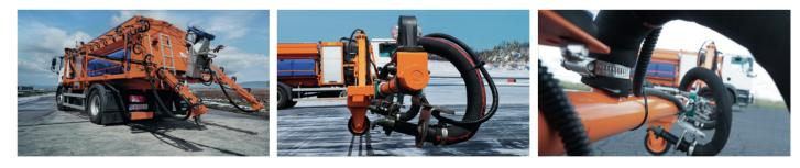
Orion Combi is an airport combination spreader of solid and liquid chemical reagents model, with spreading disc, and spreading arms, designed for de-icing treatment of airport runways, taxiways and parking areas. Works with most de-icing chemical reagents based on acetate, formic acid, glycol and urea.
